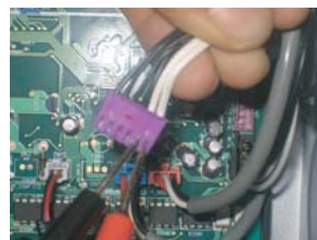
Check the resistance inverter compressor discharge temperature sensor
