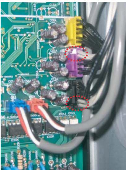
Check the resistance inverter compressor discharge temperature sensor
